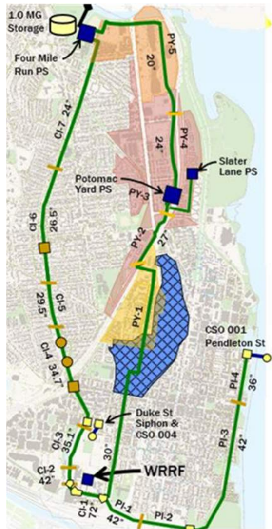
Figure 8-3: Existing Potomac Yard Sanitary Sewer Infrastructure
