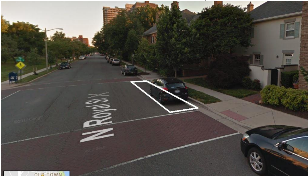
N Royal Street, looking south. White box shows where pedestrian bulbout will replace slightly less than two parking spaces on the west side of the street.
