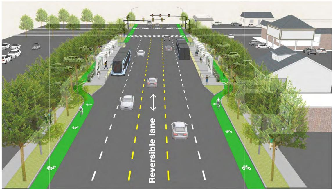
**Figure 4.31: Reversible Lane Concept with On-Street Bicycle Facility**
