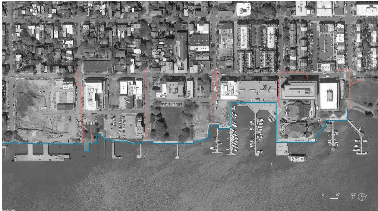
Figure 3: Existing Stormwater Infrastructure
