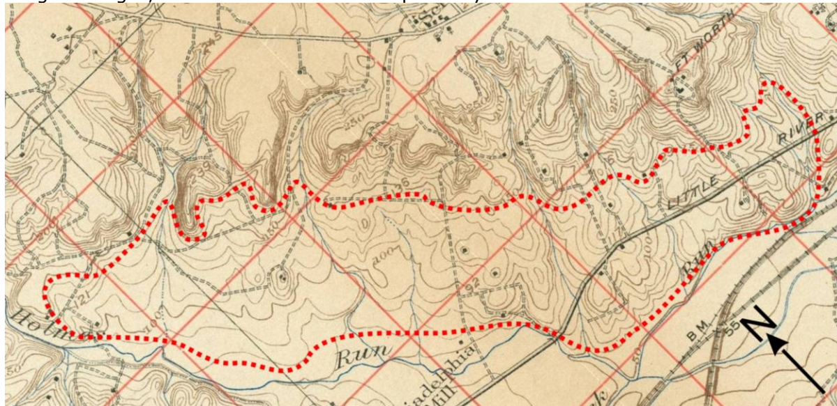
Figure 5-17. The distinctive physiography of the Seminary Valley fan (outlined by the red dotted line) and its relations to the Hospital escarpment and Holmes Run, as seen on this 1917 topographic map, which precedes widespread urbanization.
