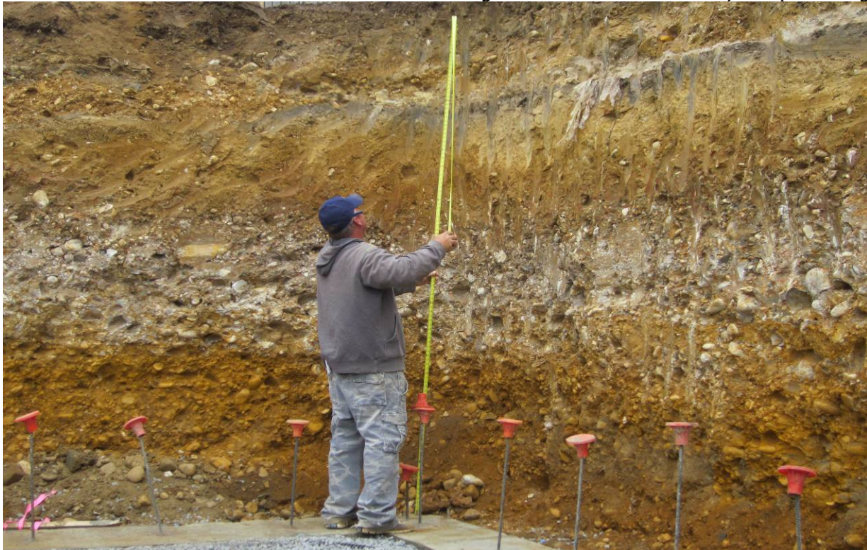
Figure 5-9. The gravel is very poorly organized, and may exhibit a crude layering or imbrication of clasts. Faint cross bedding, such as that visible to the right of the person at about waist level, is rarely seen outside of excavations. Chinquapin Village terrace, exposure 312. Photo by Rod Simmons.
