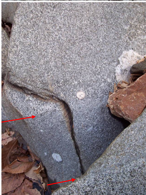
Figure 3-8. Top: Occoquon Granite is readily recognized by its "salt and pepper" texture, produced by grains of dark biotite mica within a light background of quartz and feldspar. Lower left: Sharp contacts (arrows) between coarse-grained biotite granite and finer-grained, grayer Indian Run Formation. Right: Small vein (arrow) of pink-white granite in Indian Run Formation. Dora Kelley Park above Beauregard Street. Photos by Tony Fleming.
