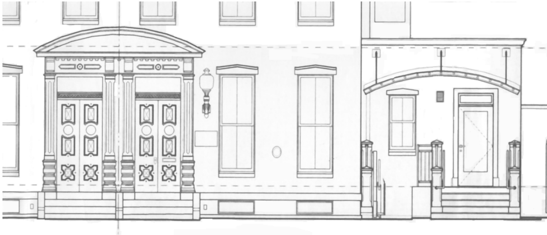
Figure 1 411 North Washington Street. New accessibility ramp uses architectural detailing from the existing historic building to comply with the Washington Street standards.
