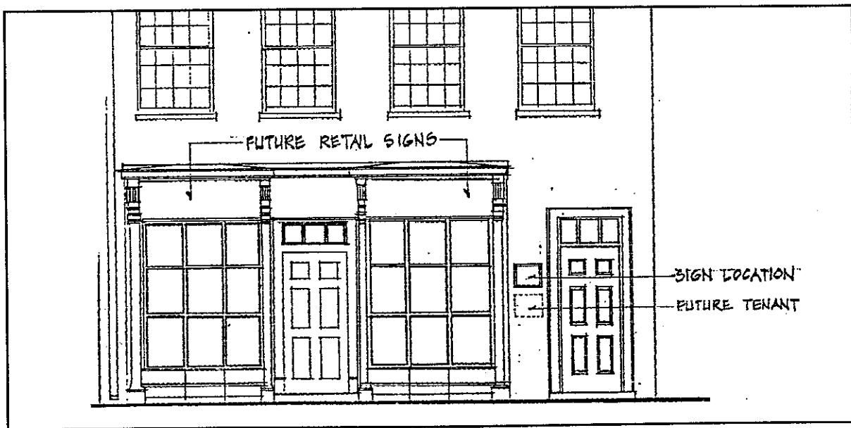
Sign plan for a building on King Street including approval of one sign and location of future signs.
