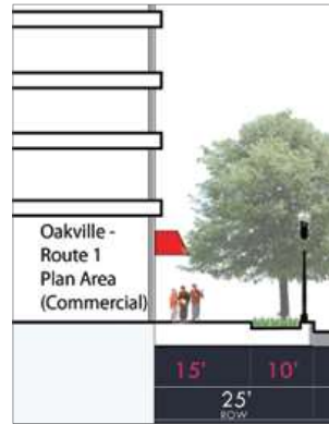
Figure 15 Route 1 Streetscape Cross-Section (Commercial)
