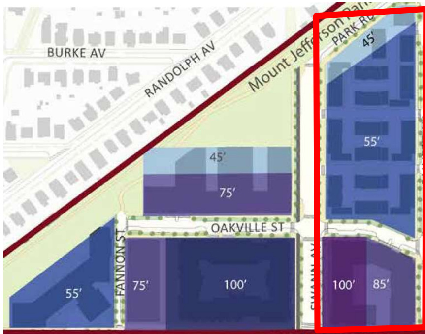
Figure 28: Minimum Building Heights
