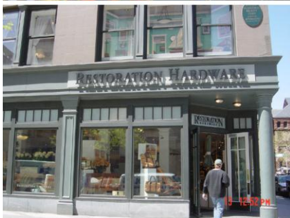
A well designed retail facade should be at least 75% transparent and should incorporate awnings as these examples in Boston, MA do.
