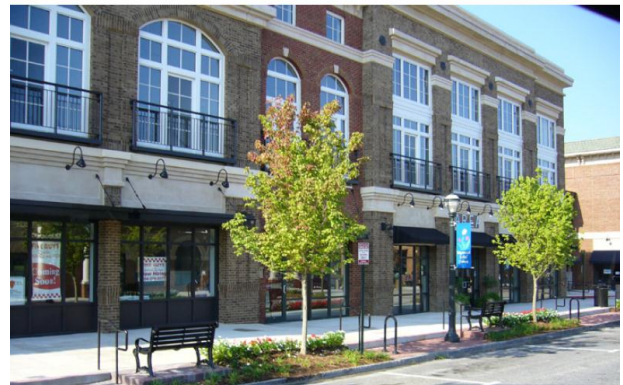
Mixed-use buildings should include a high-degree of transparency at ground floor commercial uses and a distinctly different façade treatment on upper residential floors, typically expressing bay dimensions of rooms and dwelling units. Examples shown here are in Atlanta.
