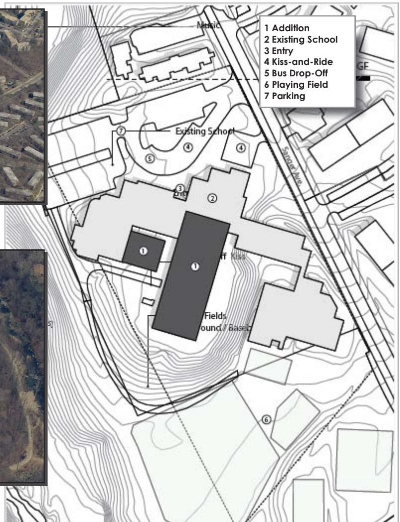
Master Plan concept showing potential enlargement of south wing and media center addition.
