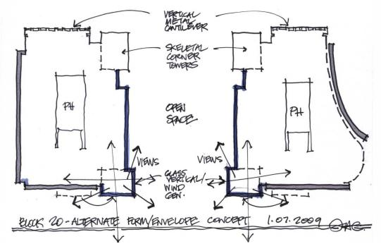
Figure 2. Design study showing tower tops integrated within building walls.
