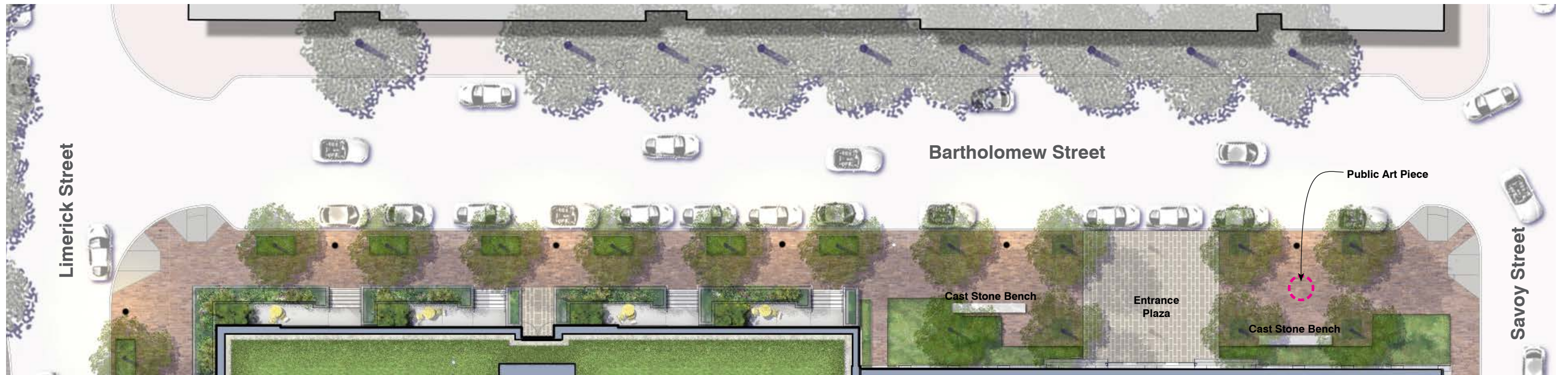
Sidewalk - (Alexandria Standard Brick) 350M, Running Bond
