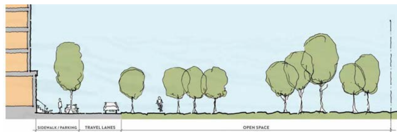
Conceptual section for shared street ("New Street B") adjacent to Potomac Yard Park.
