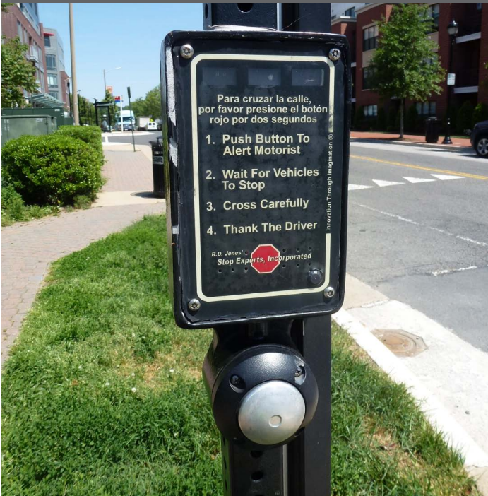
Accessible Pedestrian Signal on Mount Vernon Avenue
