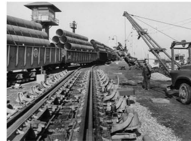
This automatic car retarder contained brakes on the tracks to slow downhill rail cars. The control tower is shown in the image background. Courtesy of George Payne.
