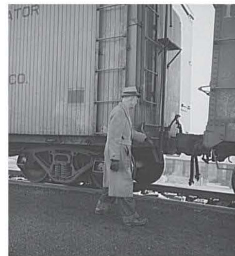
Rail cars were once uncoupled by hand on the hump by workers called car-cutters. Courtesy of the Library of Congress.
