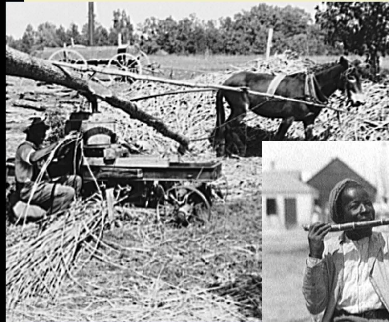
John McGinnis probably processed sugar cane using an animal-powered three-roller mill, similar to those used in 18th-century Caribbean and American plantations. This photograph shows sorghum stalks, which produce a sweet juice, being fed into a mill to make syrup in Orange County, N.C., 1939.
