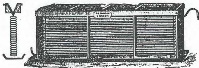
B: Improved version of Baudelot's 1856 wort cooler. Source: The Western Brewer, June 1880
