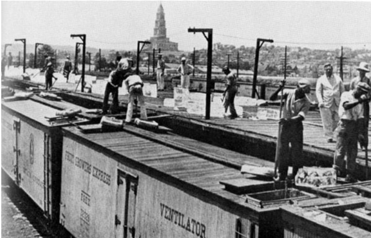
PLATE 30 Undated Photograph of Car Icing Operations; Photograph from the Del Ray Sun Web Site < http://www.delraysun.net/ >
