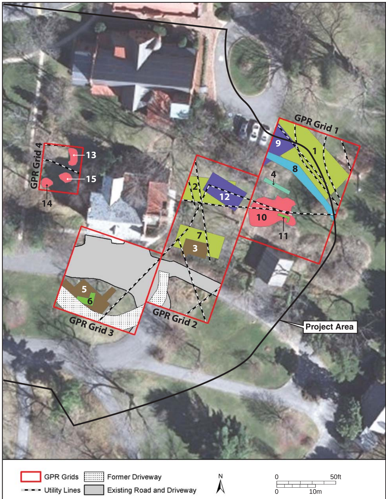
Figure 13. Numbered ground-penetrating radar anomalies within the geophysical survey areas.
