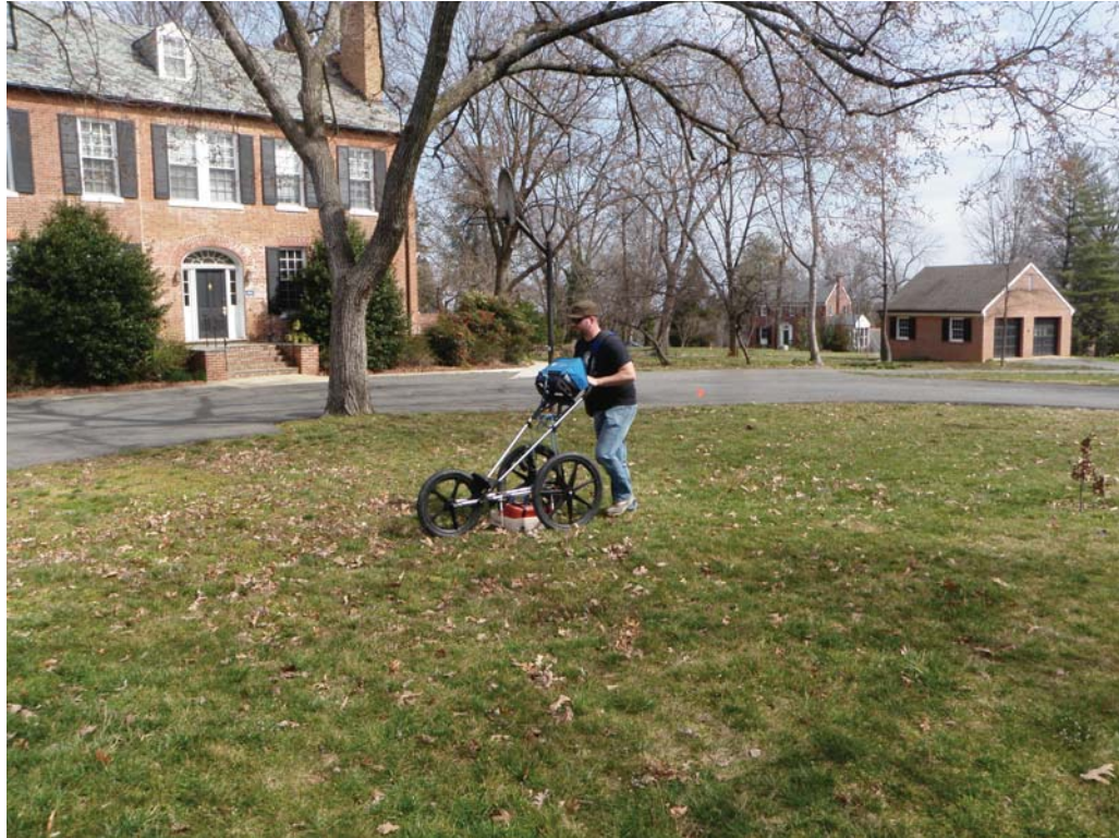
Figure 2. Geophysical Survey Systems, Inc. Ground-Penetrating Radar System used at the Virginia Theological Seminary.
