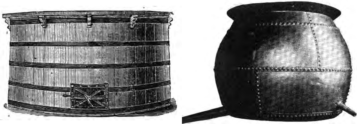
Left: A "modern" mash tun, pictured in Western Brewer of June 1880. Right: A mid-nineteenth-century copper brew kettle, similar to that which Robert Portner would have used during the Civil War, from One Hundred Years of Brewing.
