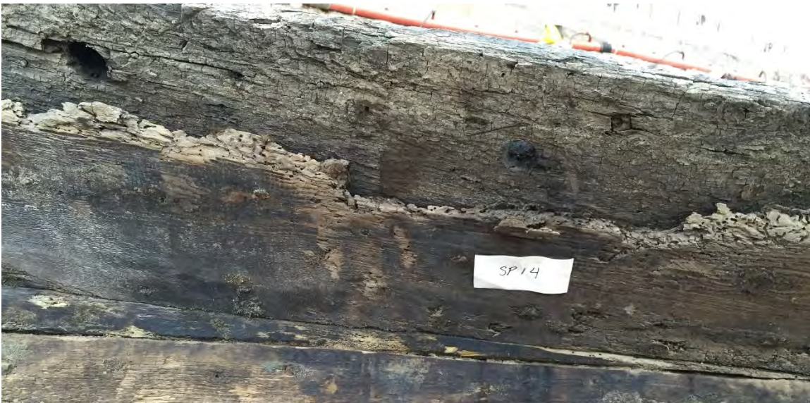
Figure 134: Feature 53, Sacrificial Planking on Keel, Showing Shipworm Damage
