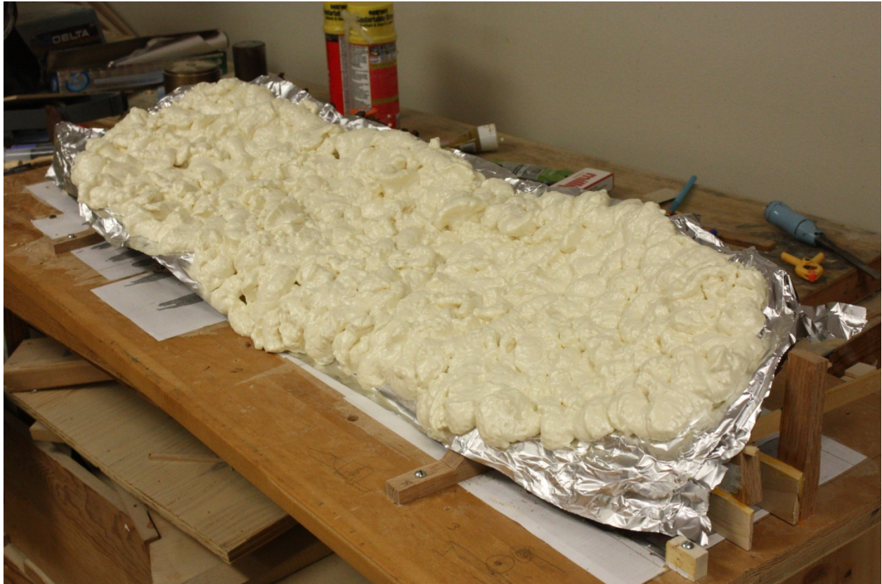
Figure 4 Completed frame model covered in Aluminum foil and rigid expanding foam. (Photo by Glenn Grieco)
