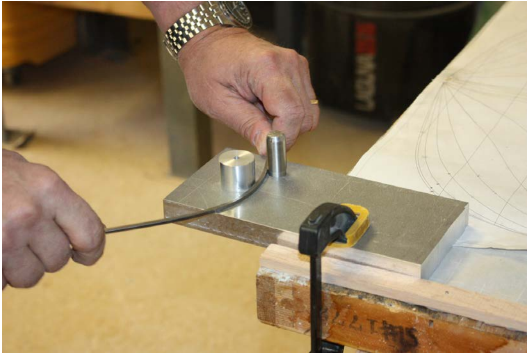
Figure 7: Using the bending jig to form one of the Indigo's frame sections (Photo by Glenn Grieco)
