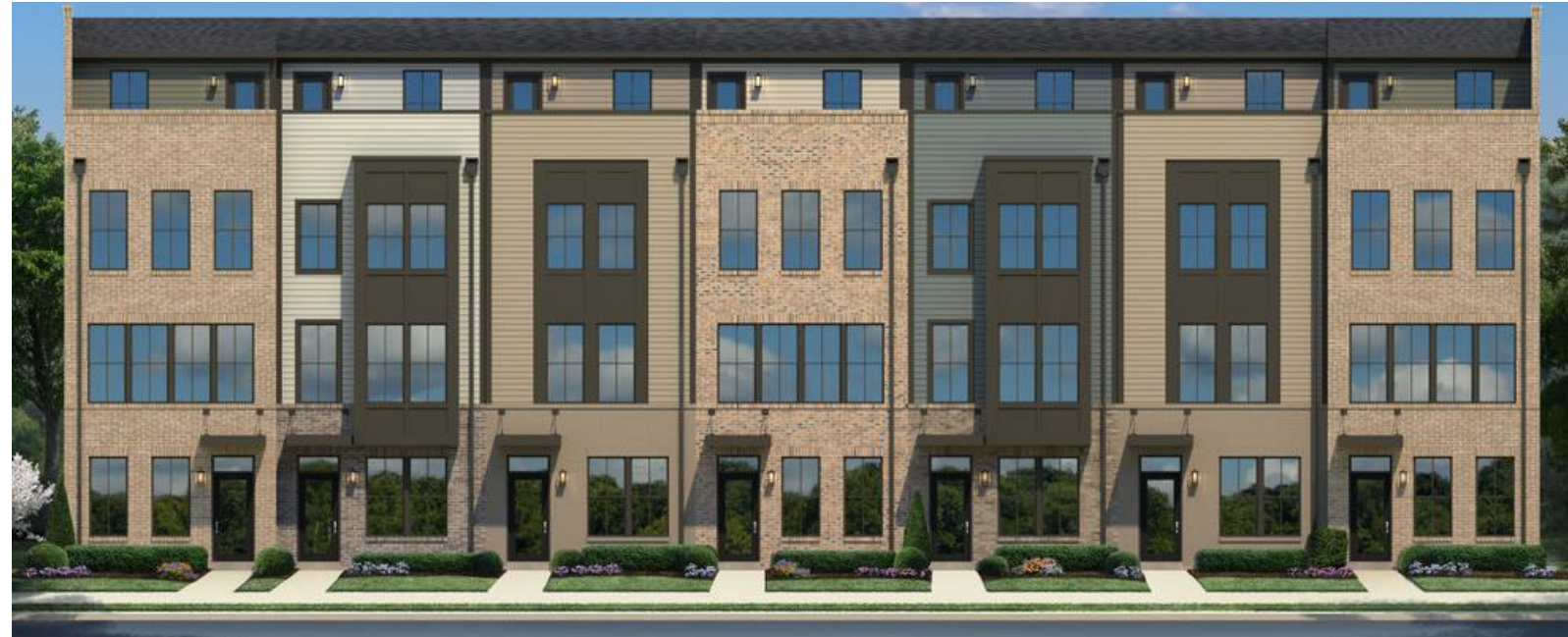
7-UNIT FRONT ELEVATION FULL BRICK FRONTS AT BUILDING ENDS AND CENTER INTERIOR UNIT OTHER UNITS PARTIAL BRICK AND SIDING
