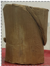
Specimen 3 Failure Sketch
