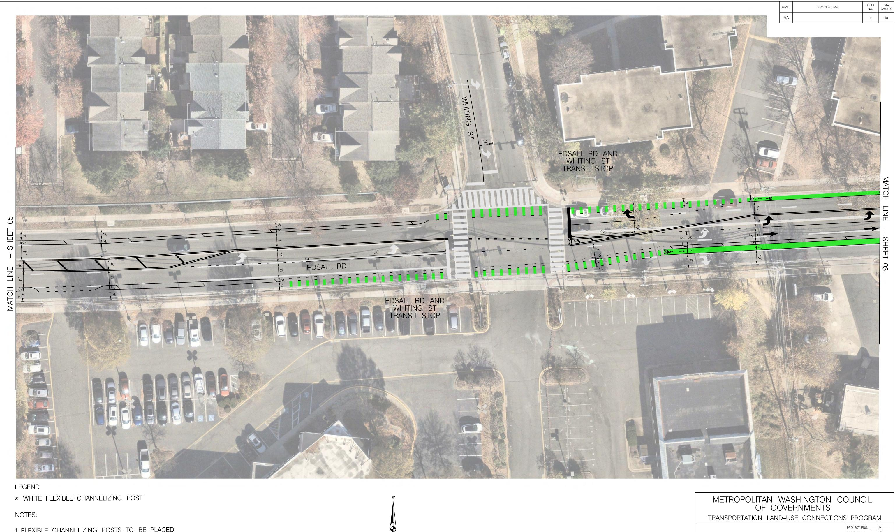
1. FLEXIBLE CHANNELIZING POSTS TO BE PLACED STRATEGICALLY TO PREVENT RIGHT TURNS FROM MINOR APPROACHES/DRIVEWAYS FROM ENTERING THE SEPARATED BIKE LANE
