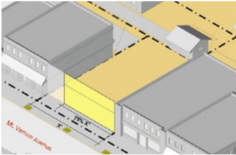
Figure 6.13 Street frontage interior site
