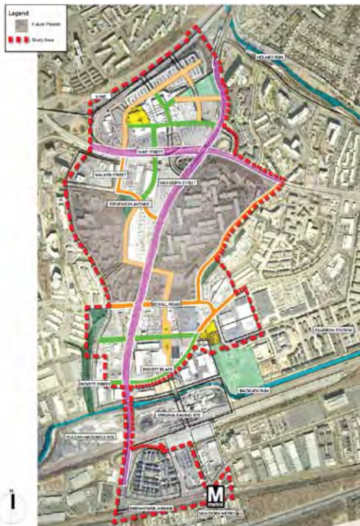
Figure 9-1. Stormwater Management Strategies. This figure illustrates the application of strategies outlined in Table 9-4 on the following page. Color codes in the table show application of appropriate strategies to streets and open spaces.
