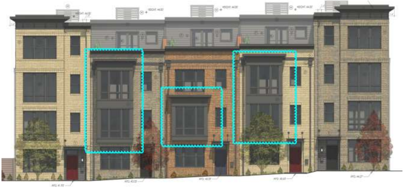
SOUTH ALFRED STREET - STREETSCAPE ELEVATION Figure 7: Encroaching bay windows on South Alfred Street.
