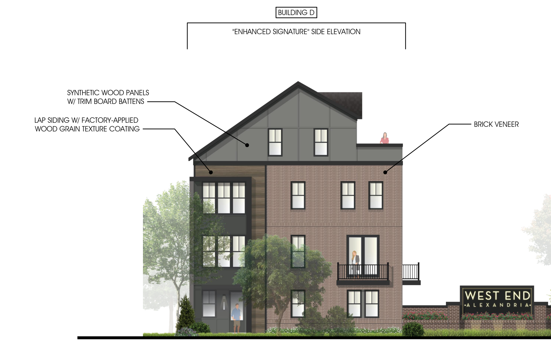
BUILDING D "ENHANCED SIGNATURE" SIDE ELEVATION 3/32" = 1'-0"
