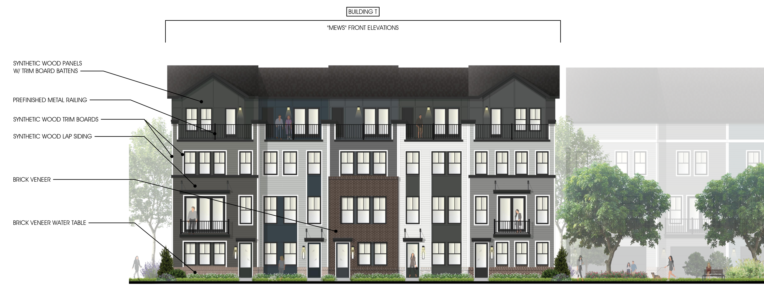
A BUILDING S "MEWS" FRONT ELEVATION 3/32" = 1'-0"
