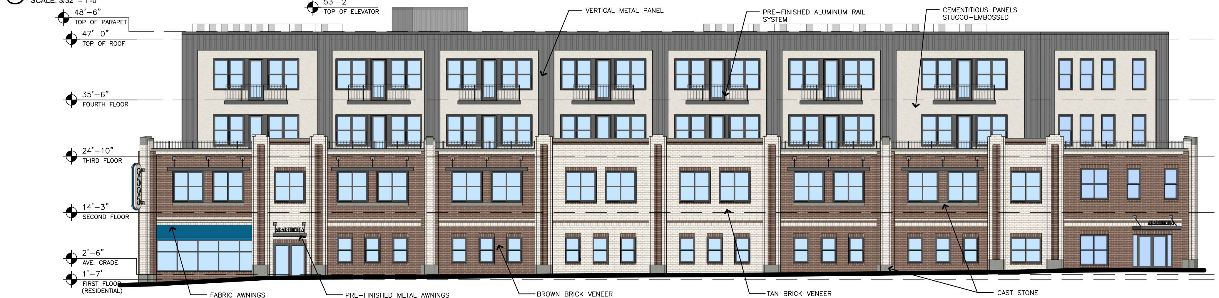
2 Mt. Ida (South) Elevation SCALE: 3/32" = 1'-0"
