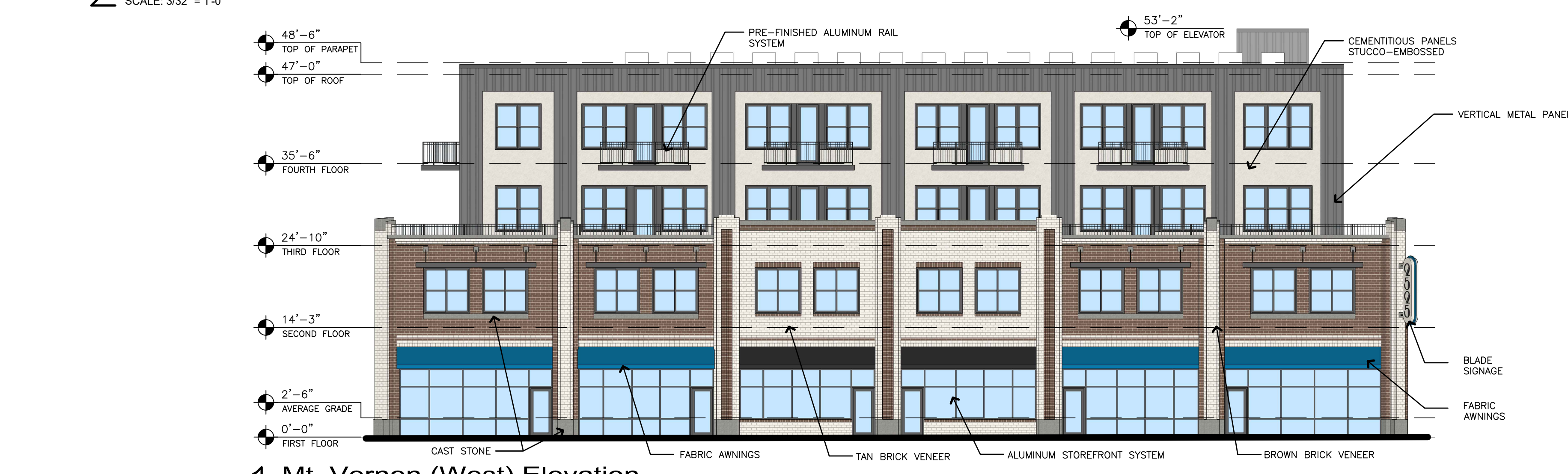
1 Mt. Vernon (West) Elevation SCALE: 3/32" = 1'-0"
