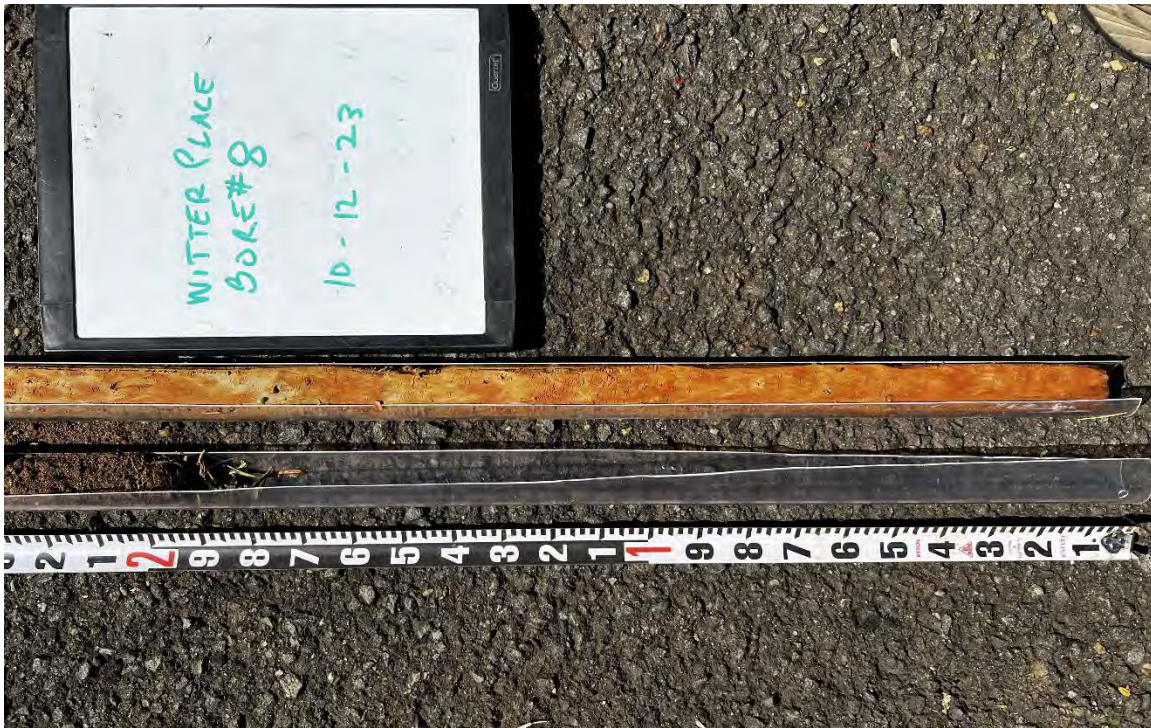
Figure 35: Soils from Test Bore B-8 Showing Truncated Substrata
