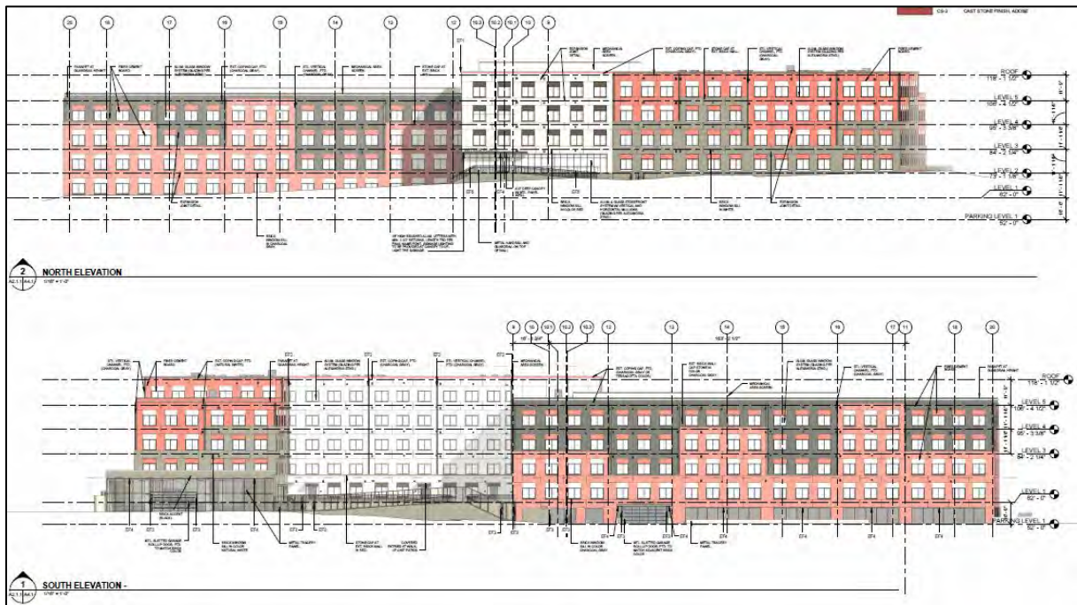
Figure 27: North and South Elevations of Proposed Development
