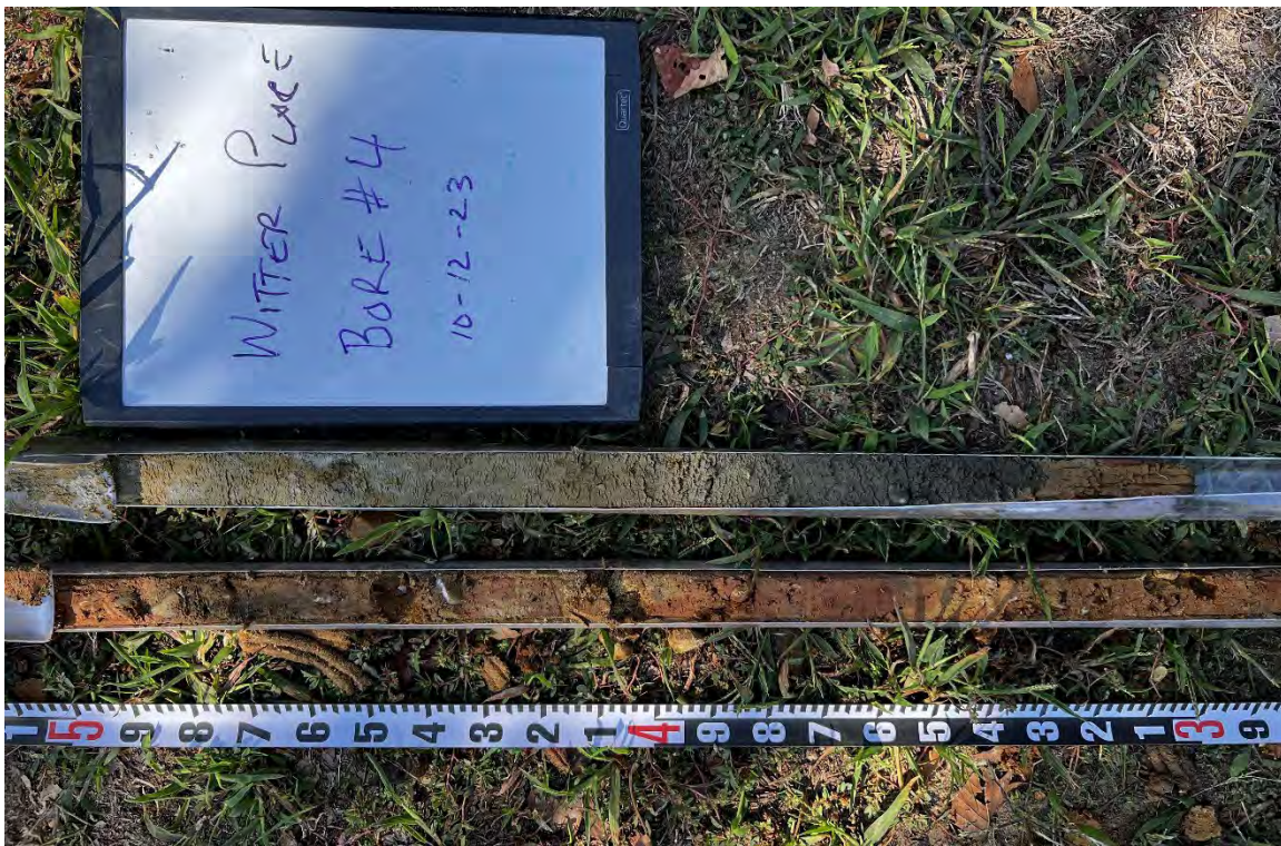
Figure 36: Soils from Test Bore B-4 Showing Apb-E-B Soil Sequence (Upper)
