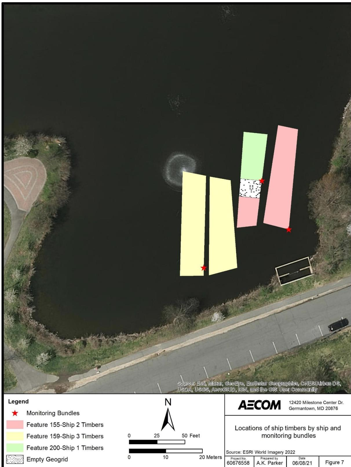
**Figure 7. Locations of ship timbers and monitoring bundles within the project geogrids.**
