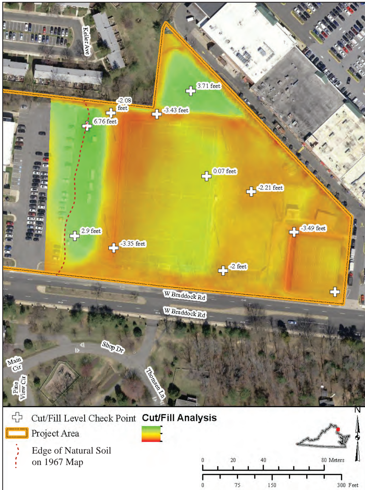
Figure 20. Estimated depth of cut/fill activity within the project area.
