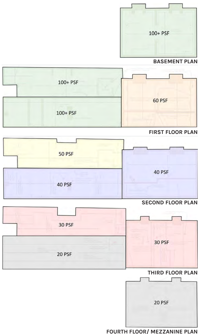
Figure 15: Structural live load capacity analysis diagrams.
