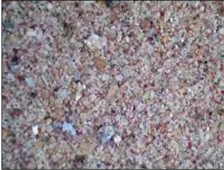
Figure 9: Sample 1 Mortar sands under simulated daylight illumination, 7.5x.
