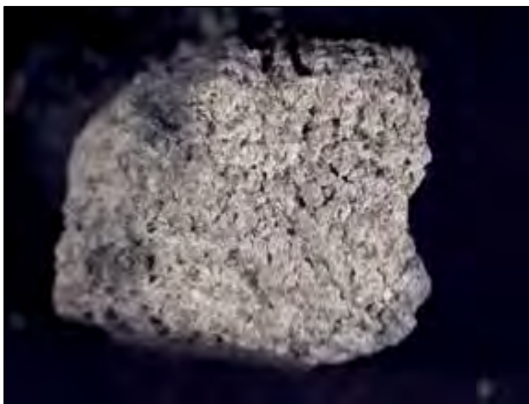
Figure 14: Sample 3 Mortar under simulated daylight illumination, 7.5x.
