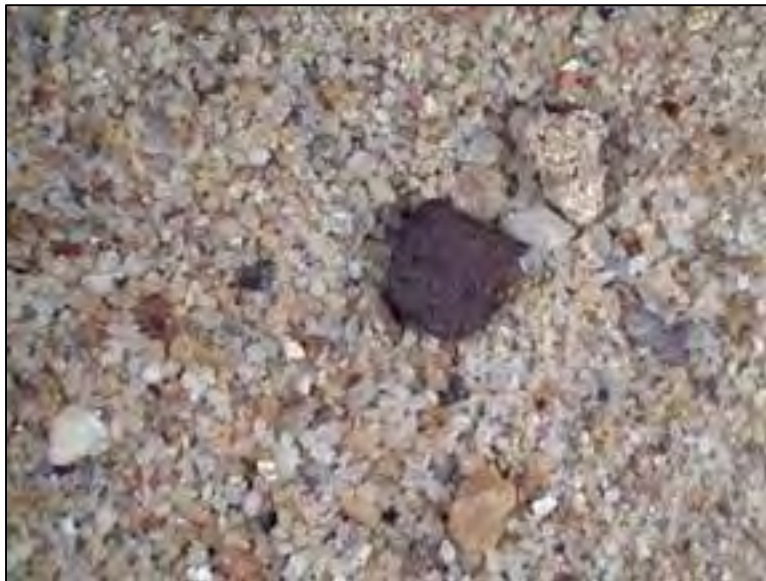
Figure 22: Sample M-6 sands under simulated daylight illumination, 7.5x.
