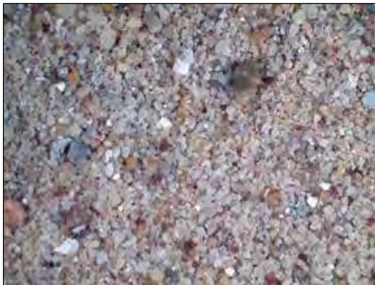
Figure 12: Sample 2 Mortar sands under simulated daylight illumination, 7.5x.
