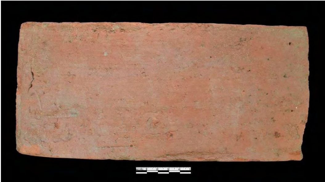
Photo 52: Brick from Feature 16a (Cistern Period) Showing the Faint Linear Strike Marks on the Surface Showing the Removal of Excess Clay During Manufacturing.
