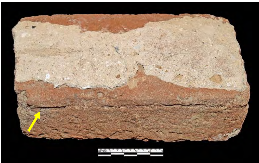
Photo 49: Brick from Feature 2, the Foundation, Showing the Linear Mold Line That Suggests a Void in the Mold Itself (Yellow Arrow). Also note the presence of shell-tempered mud mortar.
