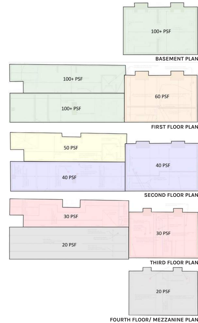
Figure 15: Structural live load capacity analysis diagrams.
